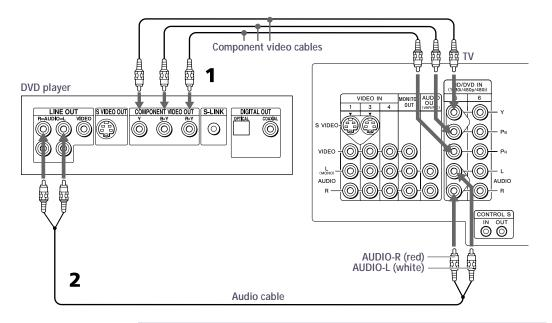
You cannot use the MONITOR OUT jacks to record the signal from any equipment connected into the Y, PB, PR jacks.
